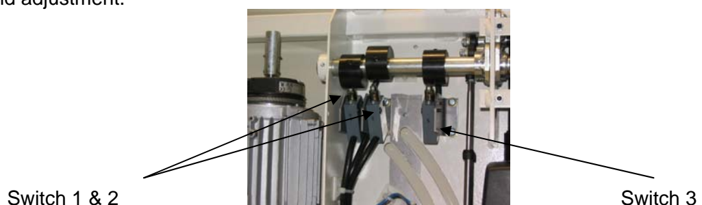
Fig.7.1a barrier arm switches
